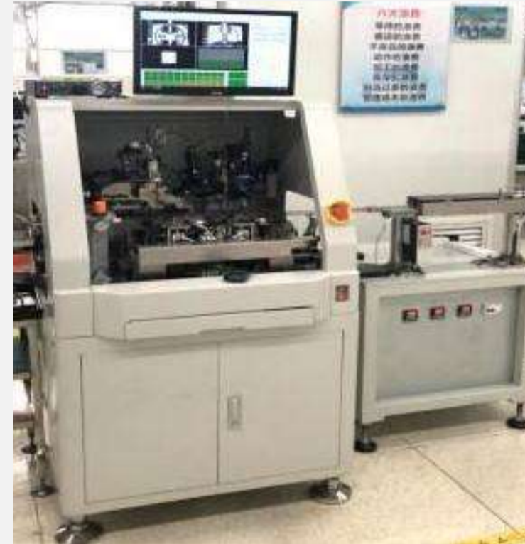
Qty: 2 Brand: Sinobonder Usage: 45 degrees glass surface mount Output: 784k/mth
