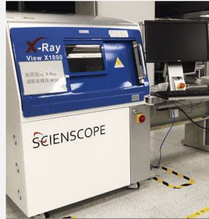
Name: X-RAY Brand: SCIENSCOPE Usage: High temp soldering inspection Output: 20.8k/mth
