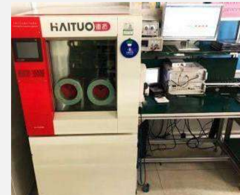
Qty: 1 Brand: HAITUO Usage: OSA-TE Hi-low temp testing Output: 8.9k/mth
