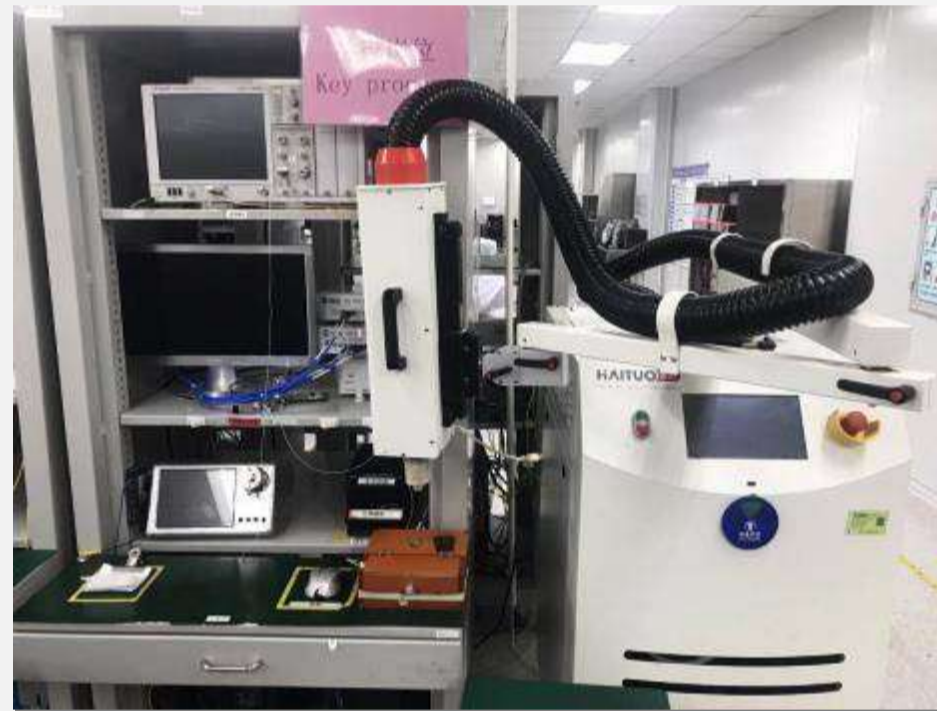
Qty: 6 Brand: HAITUO Usage: Module temp adjust Precision: \pm 1^\circ\text{C} Output: 15.6k/mth
