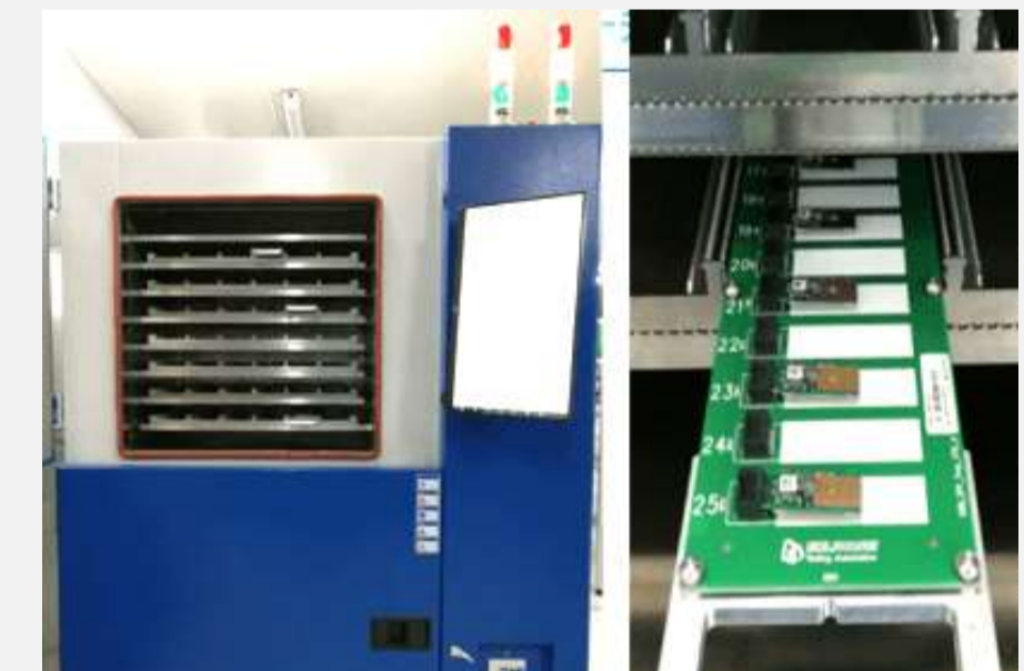
Qty: 1 Brand: home brand Usage: Weathering VCSEL&DFB Output: Weathering 26K 25G COB & 10K 100G COB at once
