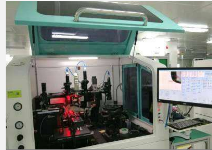
Qty: 1 Brand: ENG Usage: COB surface mount LDD&TIA die bond Precision: \leq 15\mu\text{m}@3\text{sigma} Output: 60k/mth
