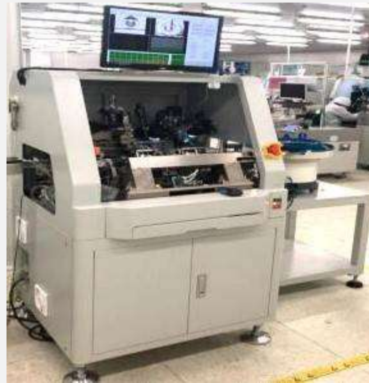
Qty: 2 Brand: Sinobonder Usage: 0 degree glass surface mount Output: 784k/mth
