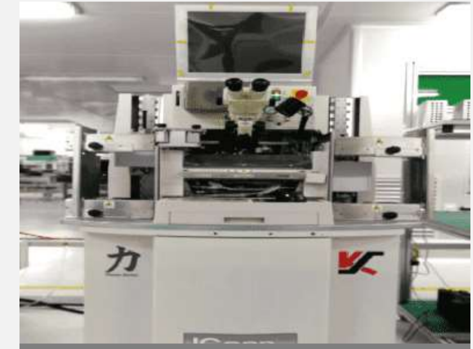
Qty: 2 Brand: KS Usage: COB soldering Precision \leq \pm 2.0\mu\text{m} Output: 80k/mth
