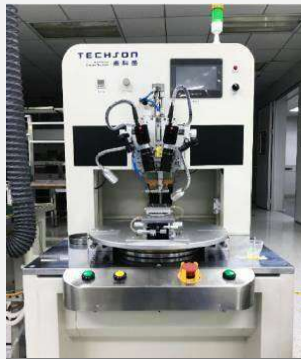
Name: high temp soldering Qty: 4 Brand: techson Usage: Soft board soldering Precision: \pm 0.1\text{mm} Output: 20.8k/mth
