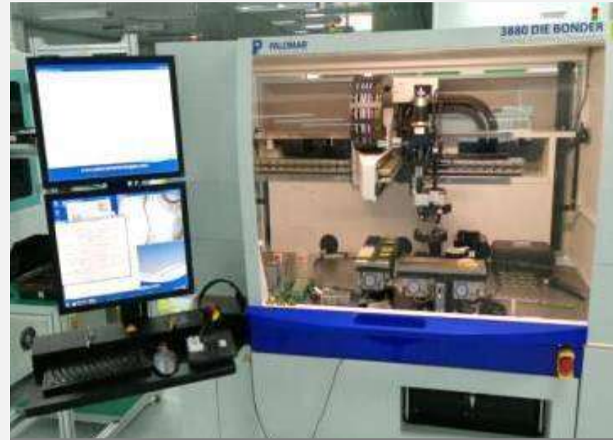
Qty: 1 Brand: PALOMAR Usage: COB surface mount, Optical chip die bond Precision: \leq 5\mu\text{m}@3\text{sigma} Output: 40k/mth
