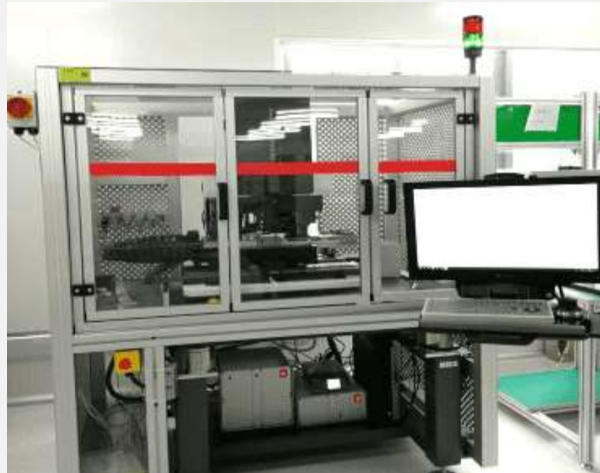
Qty: 1 Brand: Finelacer Femto Usage: COB surface mount, Soldering Precision: 0.5um Output: 10k/mth
