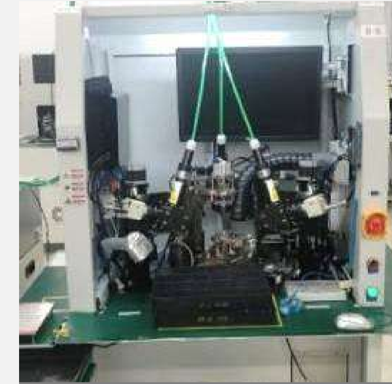
Qty: 36 Brand: Sinobonder Usage: TX coupling Precision: \leq \pm 2.0\mu m Output: 2400k/mth
