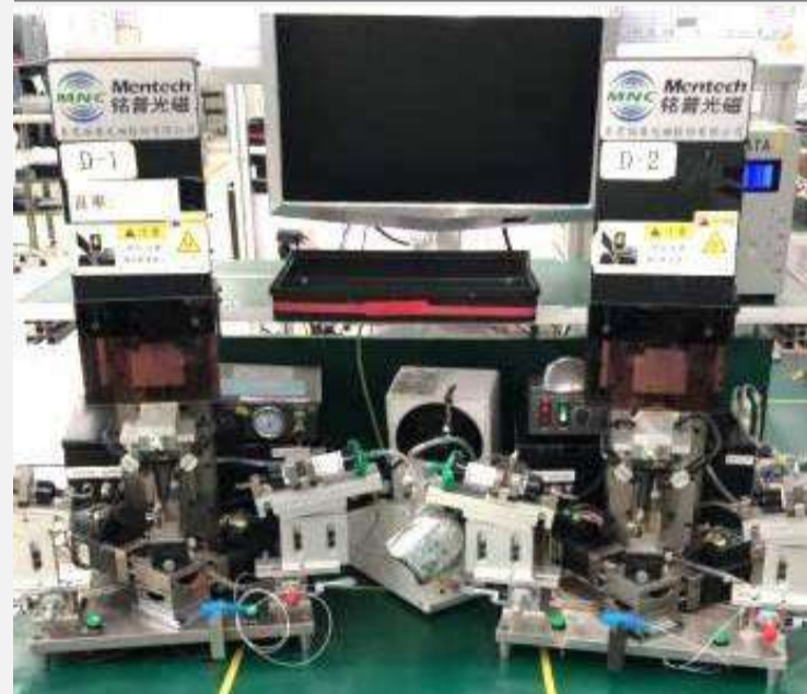
Qty: 20 Brand: home brand Usage: RX coupling Precision: \leq \pm 5.0\mu m Output: 1680k/mth
