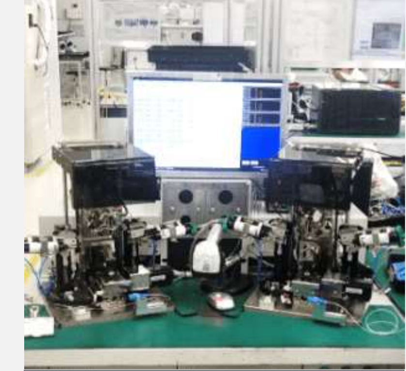
Qty: 13 Brand: Sinobonder Usage: RX coupling Precision: \leq \pm 5.0\mu m Output: 1092k/mth
