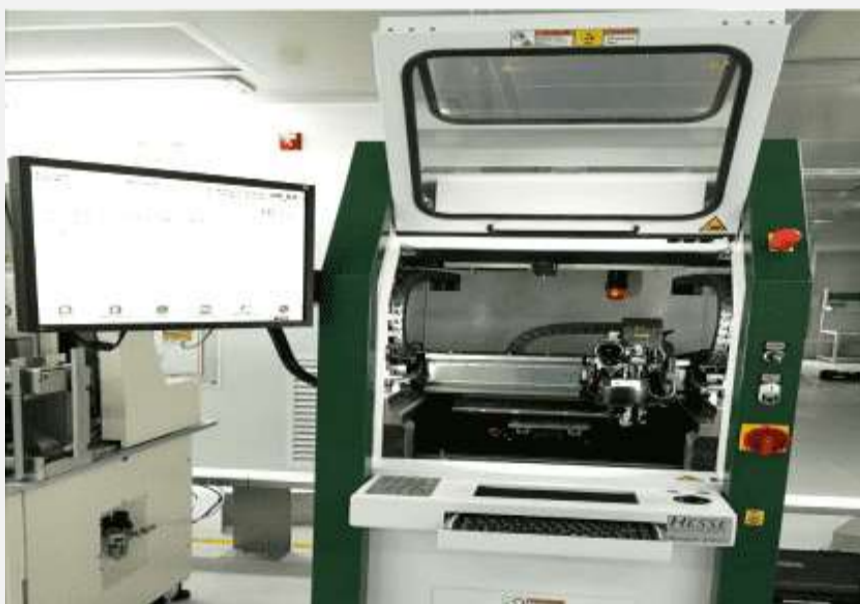
Qty: 1 Brand: HESSE Usage: COB soldering Precision: \leq \pm 3.0\mu\text{m} Output: 40k/mth
